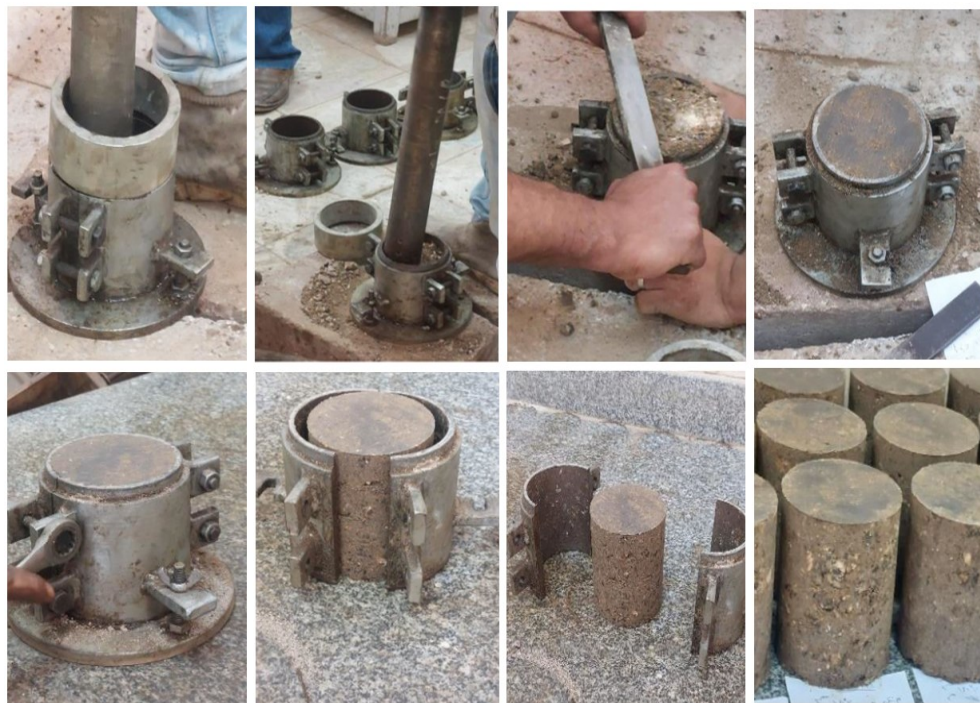
Figure 2. Specimens compacted using Proctor Molds (ASTM D1557).
