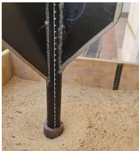
Figure 5: Measurement rulers adhered to tank walls and painted on projectiles.
