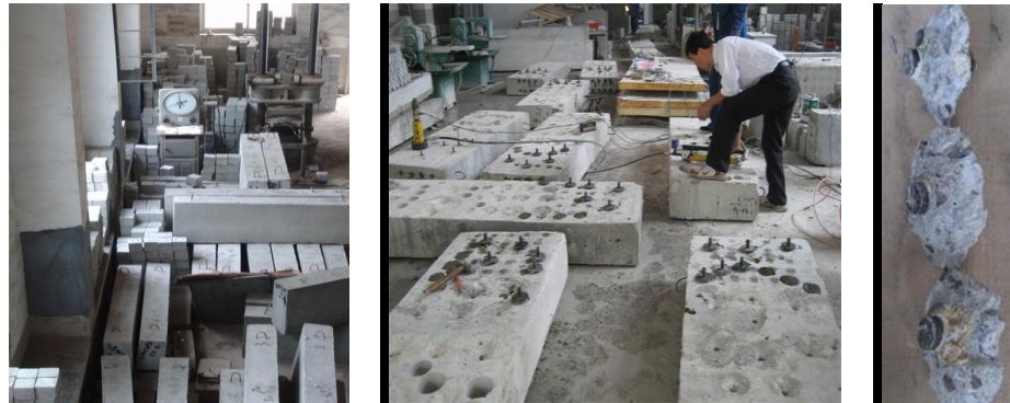
Fig.3 Specimen and frustum of anchorage pullout method
