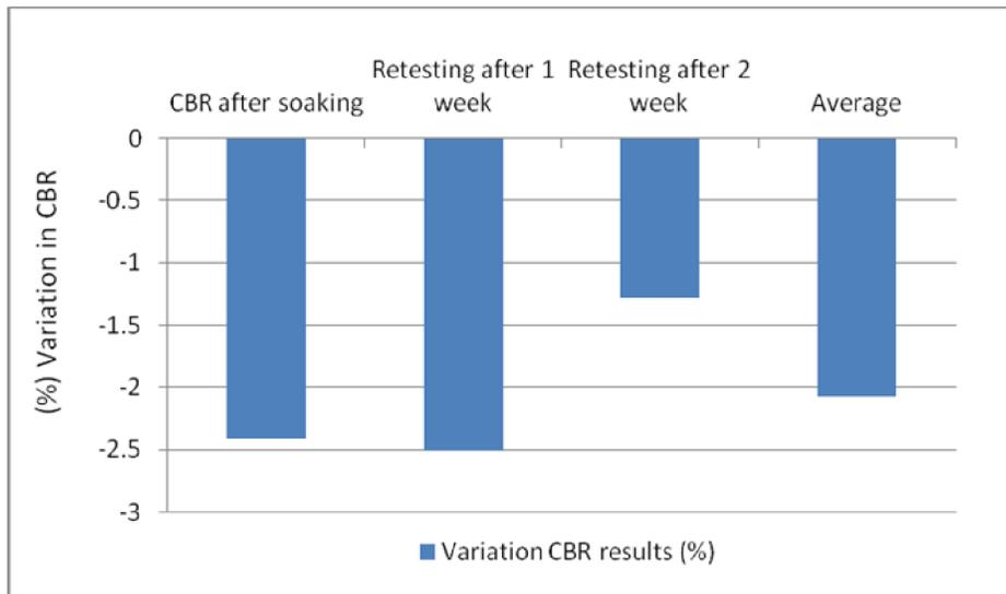
Figure (4) shows the variation in CBR values of examined crushed dolomite base course compared with the control tests (done using potable water)
