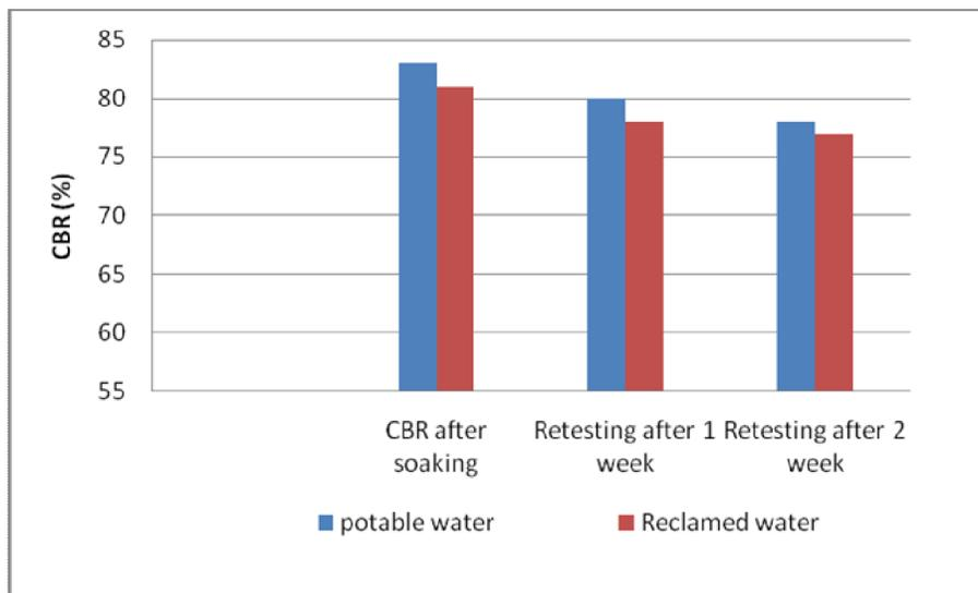
Figure (3) CBR results of the examined crushed dolomite base course material
