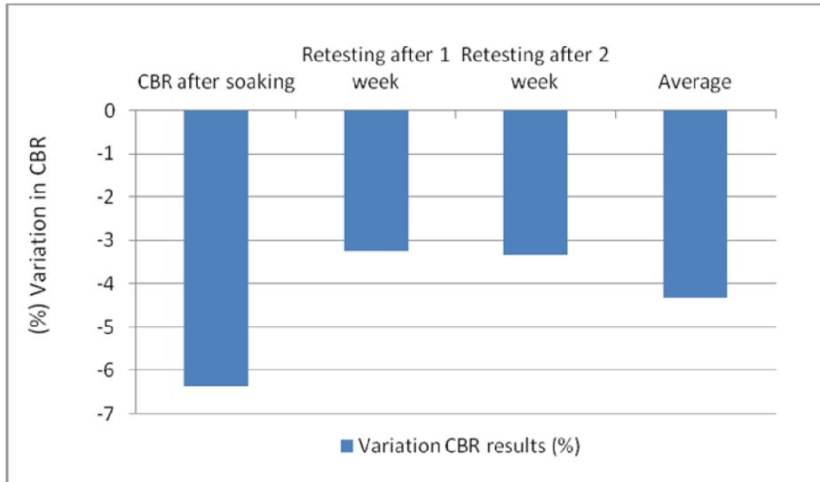
Figure (2) shows the variation in CBR values of examined crushed lime stone base course compared with the control tests (done using potable water)
