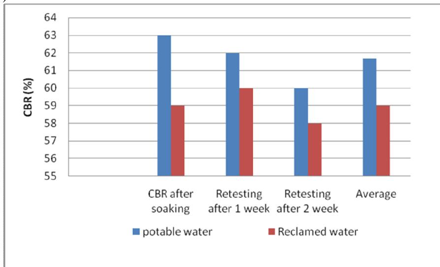
Figure (1) CBR results of the examined crushed lime stone base course material
