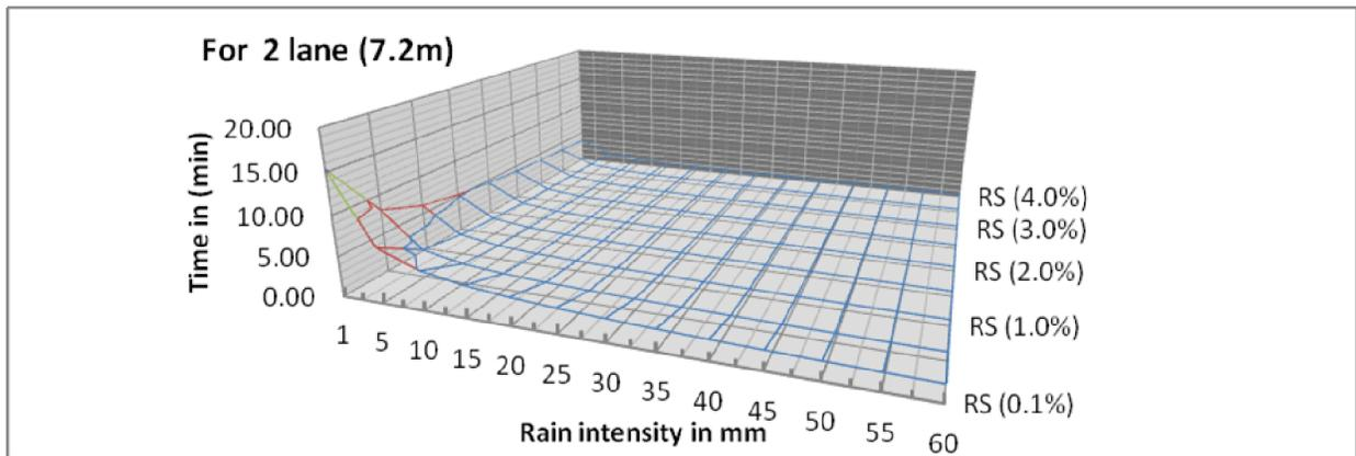
Figure (11): Shows the time of rains remains on the road surface consist of 2 lanes with manning coefficient 0.016 with different side slope (RS) and rain intensity.
