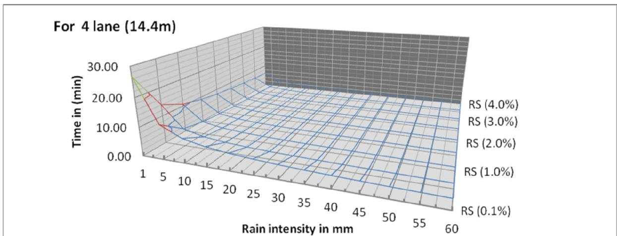
Figure (13): Shows the time of rains remains on the road surface consist of 4 lanes with manning coefficient 0.016 with different side slope (RS) and rain intensity.
