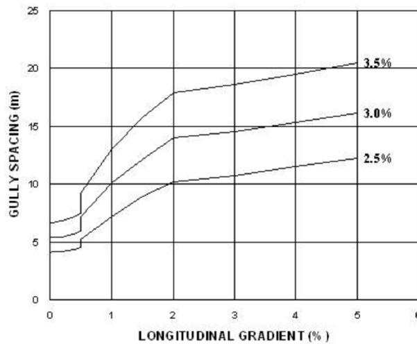
Figure (1) the effect of longitudinal gradient on gully spacing
