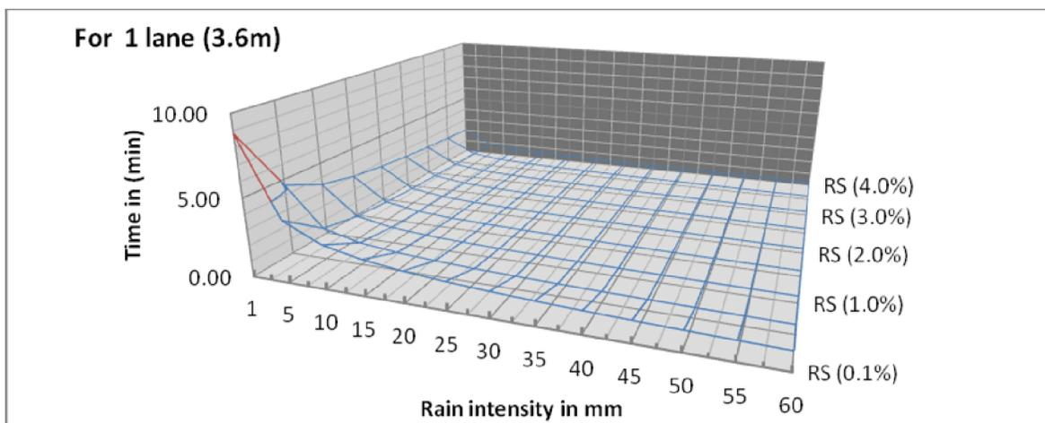
Figure (10): Shows the time of rains remains on the road surface consist of 1 lane with manning coefficient 0.016 with different side slope (RS) and rain intensity.
