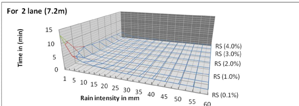
manning coefficient 0.013 with different Cross slope (RS) and rain intensity.
