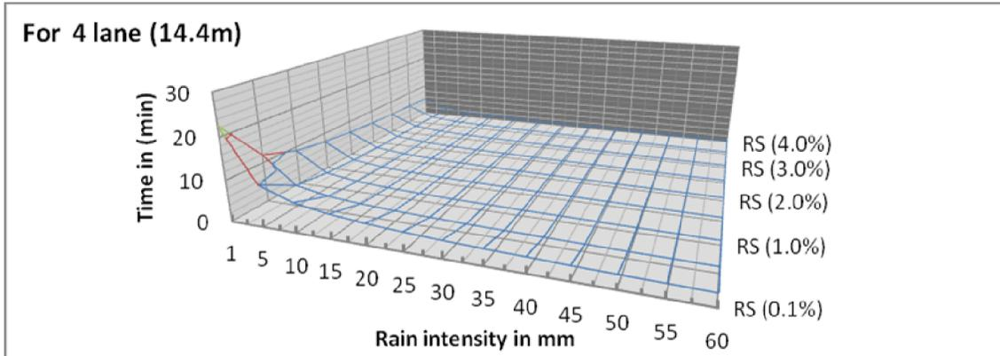
Figure (8): Shows the time of rains remains on the road surface consist of 4 lanes with manning coefficient 0.013 with different side slope (RS) and rain intensity.
