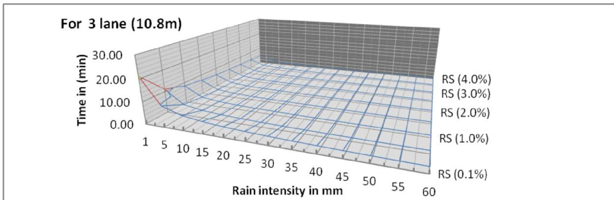
Figure (12): Shows the time of rains remains on the road surface consist of 3 lanes with manning coefficient 0.016 with different side slope (RS) and rain intensity.
