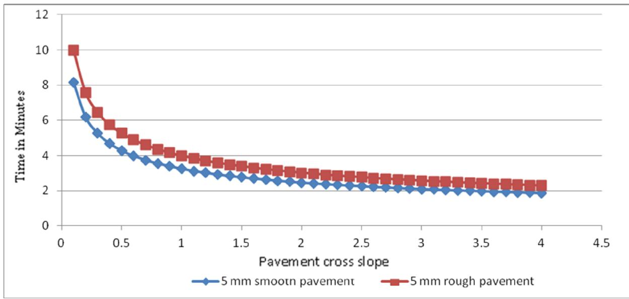
Figure (21) comparison between smooth and rough pavement drainage
