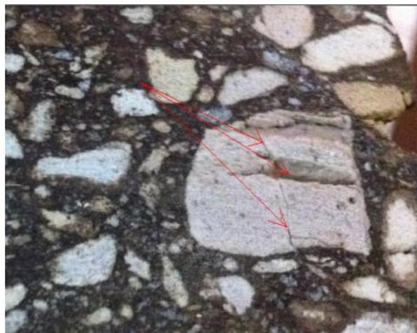
Figure (16) surface crack appears in the surface of the specimens
