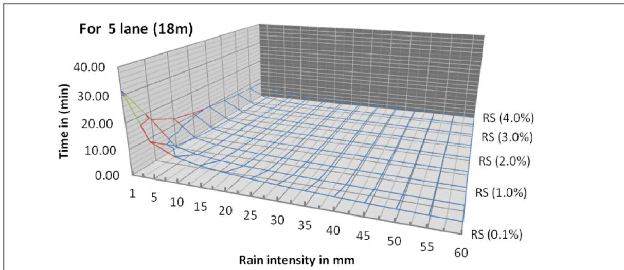
Figure (14): Shows the time of rains remains on the road surface consist of 5 lanes with manning coefficient 0.016 with different side slope (RS) and rain intensity.
