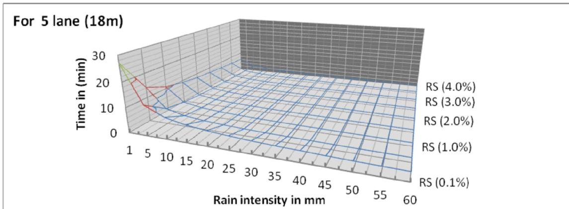
Figure (9): Shows the time of rains remains on the road surface consist of 5 lanes with manning coefficient 0.013 with different side slope (RS) and rain intensity.
