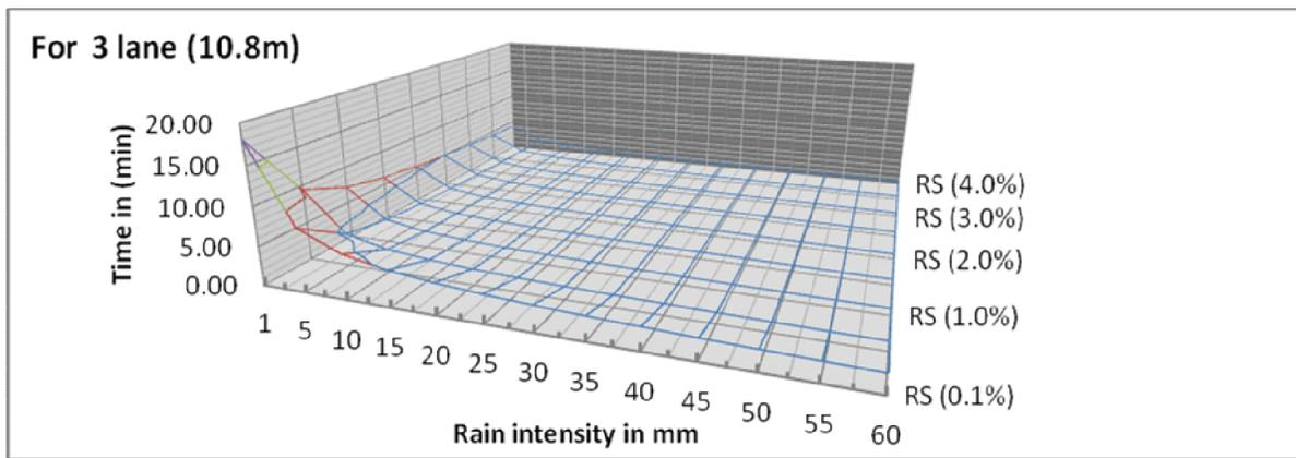
manning coefficient 0.013 with different side slope (RS) and rain intensity.
