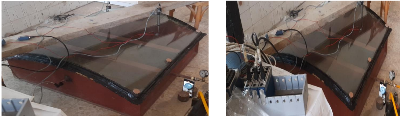
Figure 5: The position of strain gauges and displacement transducer
