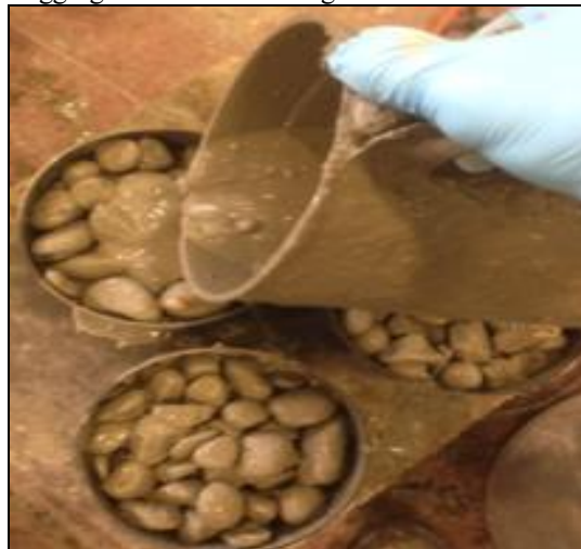
Fig. (1) TSC placing technique
