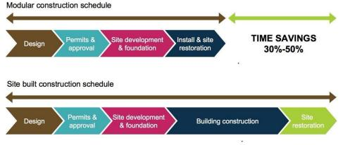
Fig.(1) Comparison between schedule of modular construction and traditional construction
