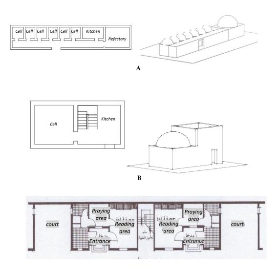
Fig. 8. Different cells design. "A" Father Pachomius total Cenobitic cell design (plan, and perspective). "B" Father Anthony prototype solitary cell in Kellia (plan, and perspective). "C" Abu Makâr cell plan [1], analyzed by Author .
