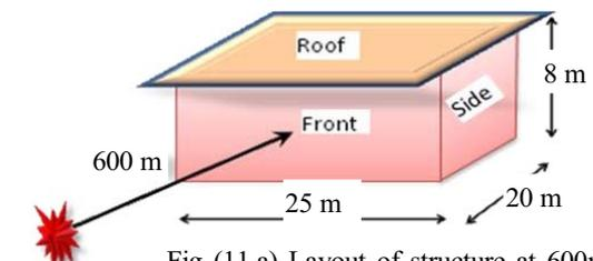
Fig (11.a) Layout of structure at 600m from 200Kt weapon yield
