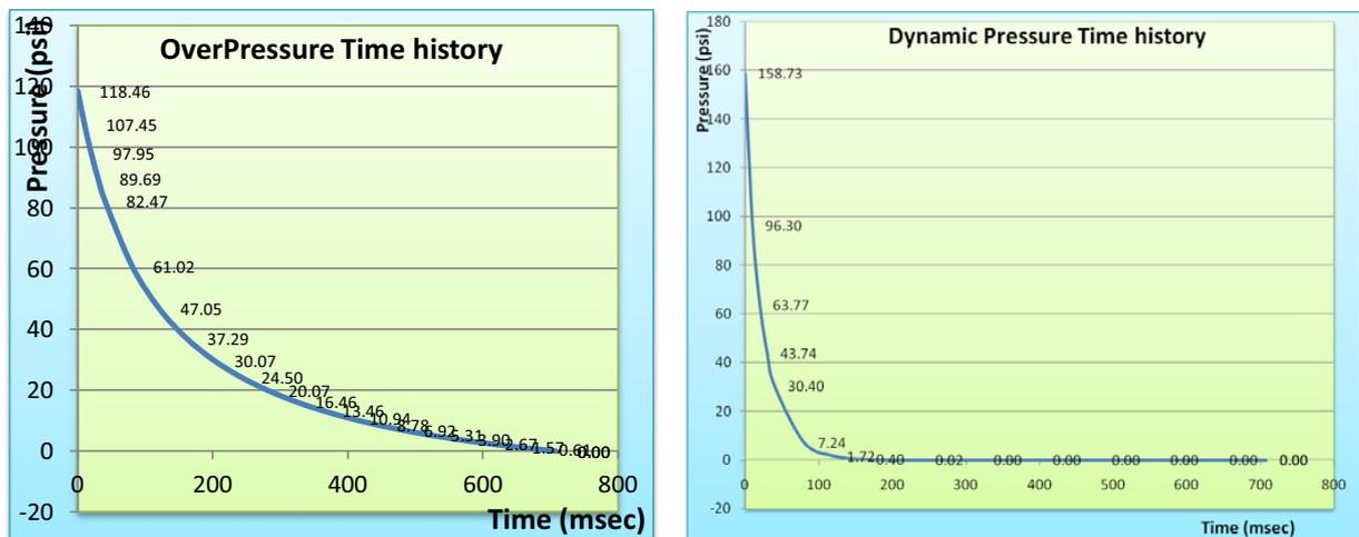
Fig (11.b) Over-pressure and Dynamic Pressure resulted from 200Kt at 600 m
