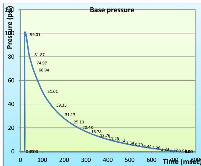
Fig (12.c) Loads on base of buried structure
