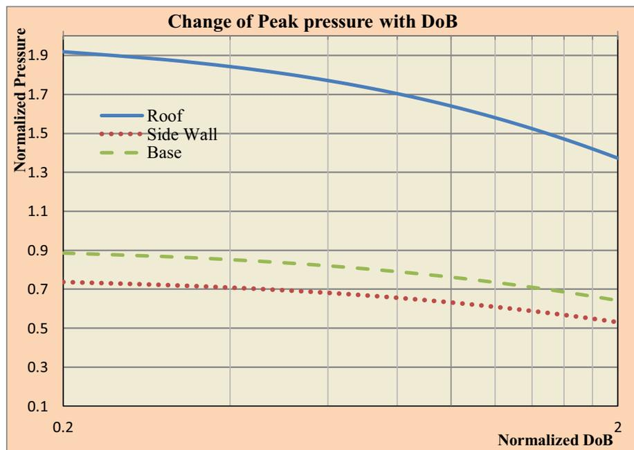
Fig (13) effect of depth of burial on peak loading on roof, side and base of buried structure
