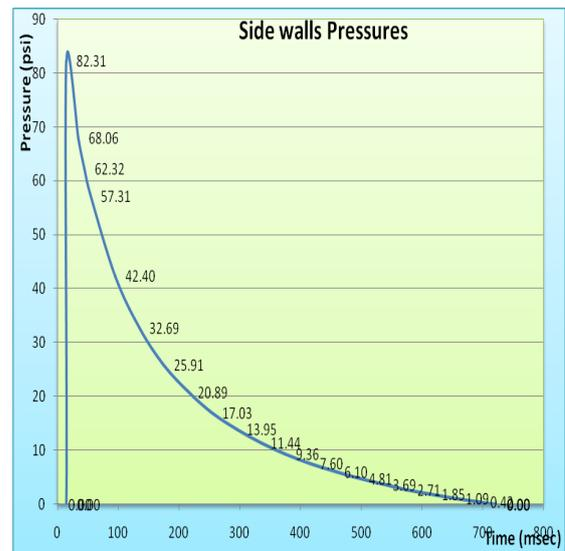
Fig (12.b) Loads on side walls of buried structure
