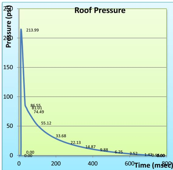
Fig (12.a) Loads on roof of buried structure
