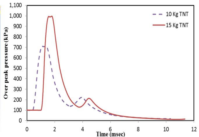
Fig (8) Loads on target from different charges at 4 m
