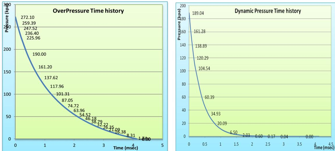
Fig (9) Over-pressure and Dynamic Pressure resulted from 15 kg at 4 m
