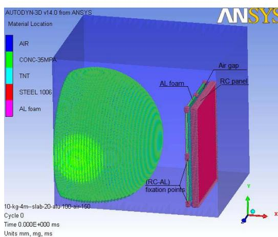
Fig (7) the boundary conditions, air medium and explosion sphere.
