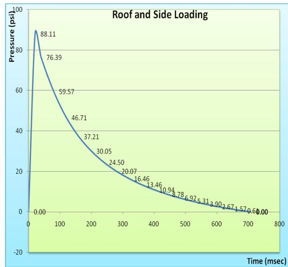
Fig (11.d) Loads on roof and sides
